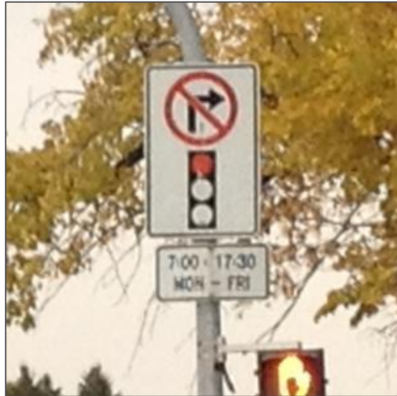
Example of No Right Turn on Red sign at intersection near school in Winnipeg. Note time restrictions (no turns during school hours).
